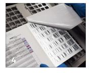
With the adhesive side facing down, orient the adhesive panel over the blister in the SynMed tray while keeping the grid panel in its folded position (5a). Align the cut marks on the grid panel with the alignment marks on the SynMed tray to ensure the panel is positioned accurately (5b).
