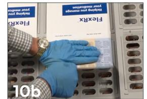
Using the roller, in a horizontal and vertical motion, apply firm, consistent pressure over the entire blister and spine of the cover to ensure that a solid seal is achieved across the surface. (11)
