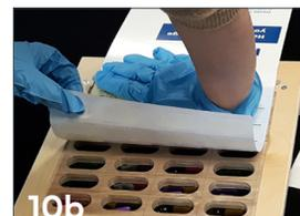
Using the roller, in a horizontal motion, apply firm, consistent pressure over the entire blister and spine of the cover to ensure that a solid seal is achieved across the surface. (11)
