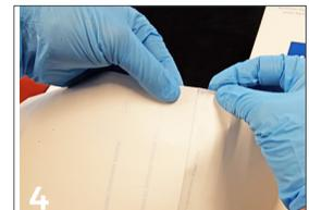
Locate the perforation above the top row of cavities and fold along this perforation, so the top part of the label meets the bottom part of the label. (5)
