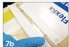
With the folded edge of the label closely aligned to the perforation on the blister, steady the positioning of the label in the middle of the tray with one hand, and then use the other hand to fold back the top part of the label toward the tray (8a). Firmly run your finger over the adhesive area on the label to join the spine of the cover to the top flange of the blister (8b)
